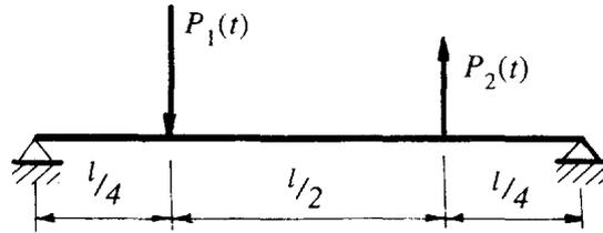
Fig. 3. The simply-supported beam under the excitation forces.
