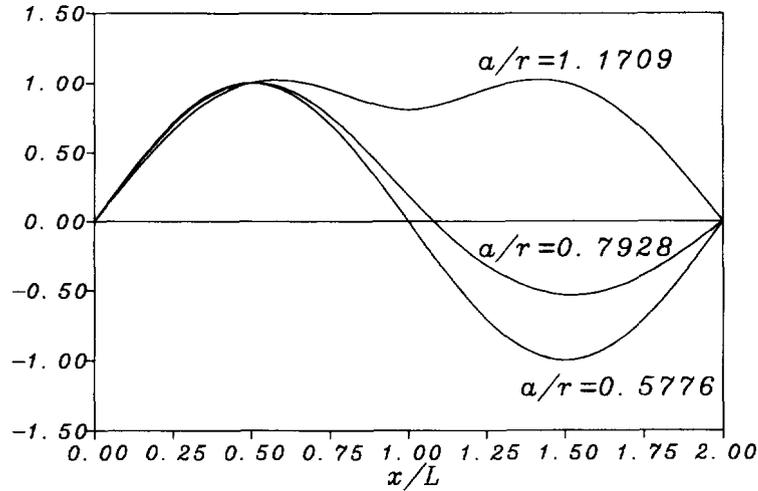
Fig. 9. The shape of "nonlinear" mode of vibration associated with the curve 3 in Fig. 7.
