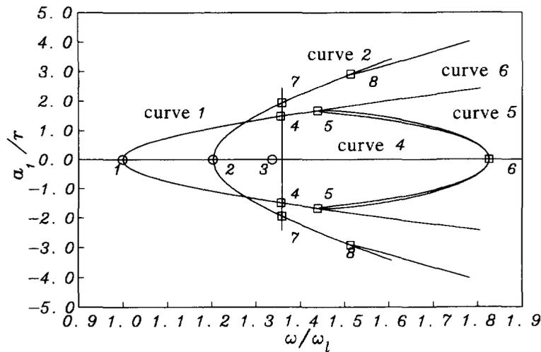
Fig. 13. The backbone curve for two span beam on the elastic support and  $kL^3/EK = 240$ .
