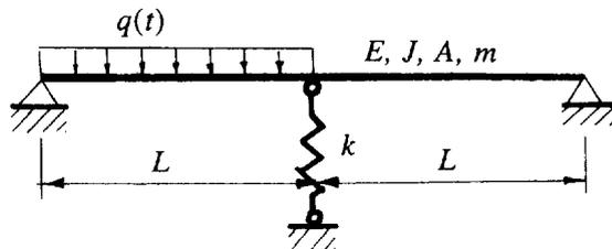
Fig. 6. The two span beam on the elastic support.
