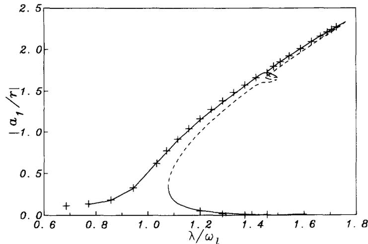
Fig. 4. The resonance curve for the simply-supported beam  $c/2\omega = 0.005$ .
