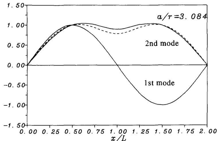
Fig. 8. Comparison of linear and "nonlinear" modes of vibration.
