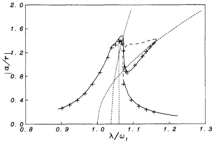
Fig. 10. The response curve for two span beam on the elastic support  $p = q/mr\omega_1^2 = 0.05$ .
