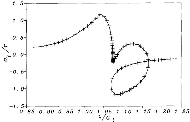
Fig. 11. Comparison of non-dimensional amplitude  $a_1/r$  for the one and two harmonics solutions.
