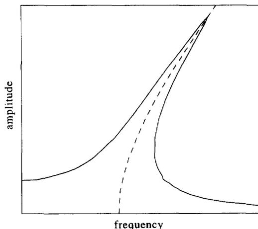
Fig. 1. The typical backbone curve (the dashed line) and the response curve (the solid line).
