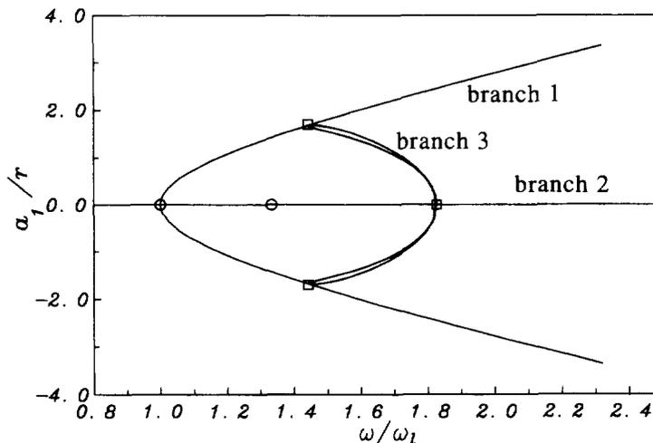
Fig. 2. The complete backbone curve of simply-supported beam.
